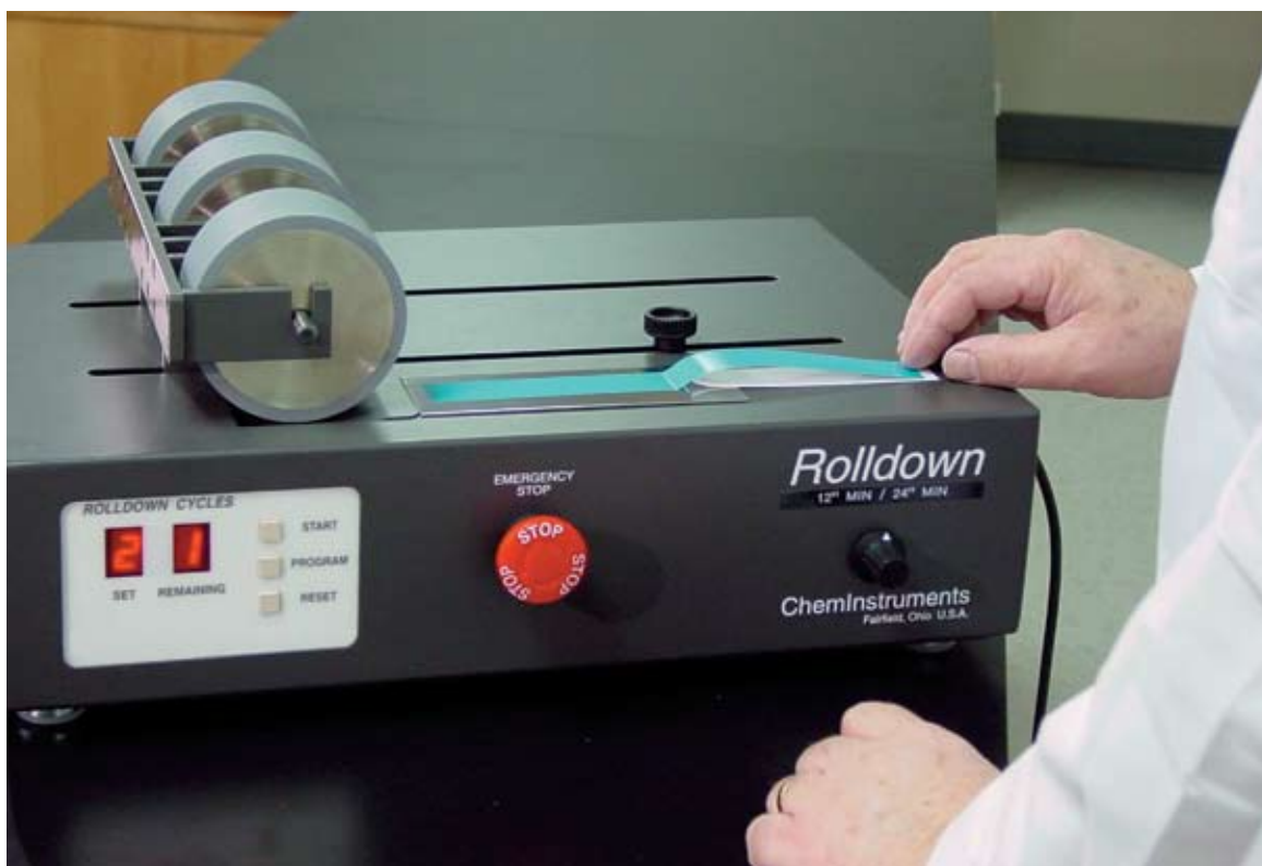
Figure 2. Mechanical roll down unit.
