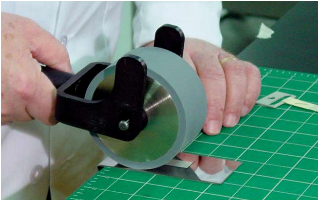
Figure 5. Sample preparation for shear adhesion hand roll down.
