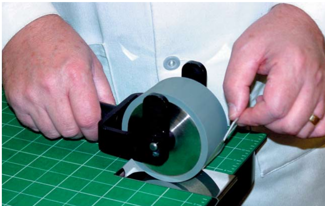
Figure 1. Controlled roll down shear adhesion sample preparation.
