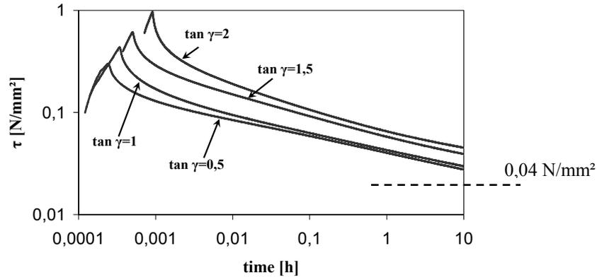
**Figure 3.** Stress relaxation from different initial strain values, acrylic pressure sensitive tape, d=1,1 mm
