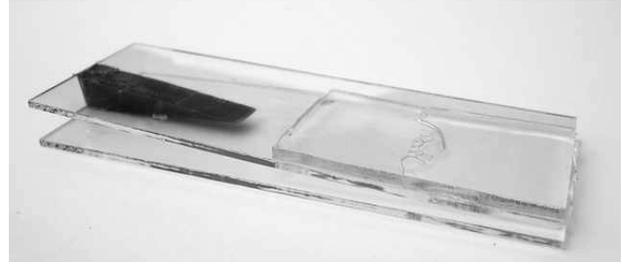
**Figure 8.** Double cantilever wedge test specimen, glass slides bonded with acrylic pressure sensitive adhesive
