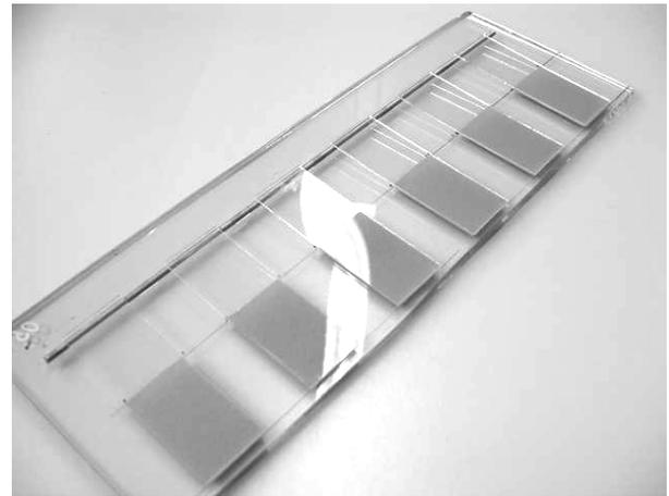
**Figure 9.** Single cantilever wedge test specimen, glass slides bonded with acrylic pressure sensitive adhesive
