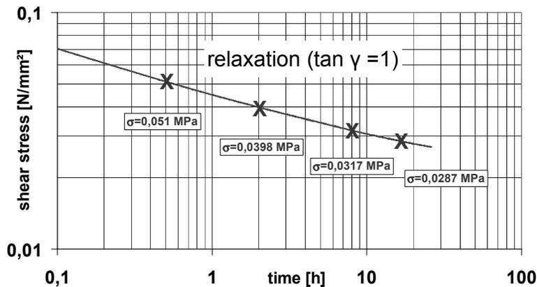
**Figure 4.** Relaxation data for aluminum lap shear specimens bonded with a 1.1 mm acrylic tape, 23 °C. The results of four corresponding creep experiments applying the time dependent load values from Fig. 4 prove that the predicted strain limit of  $\tan \gamma = 1$  was not exceeded in either one of the creep tests
