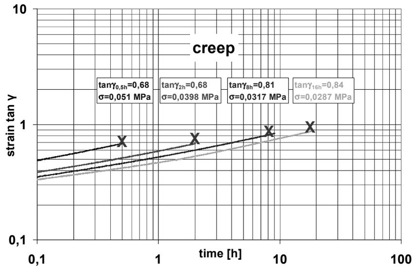
**Figure 5.** Results of creep experiments under static stress at ambient temperature corresponding to load values extracted from Fig. 4
