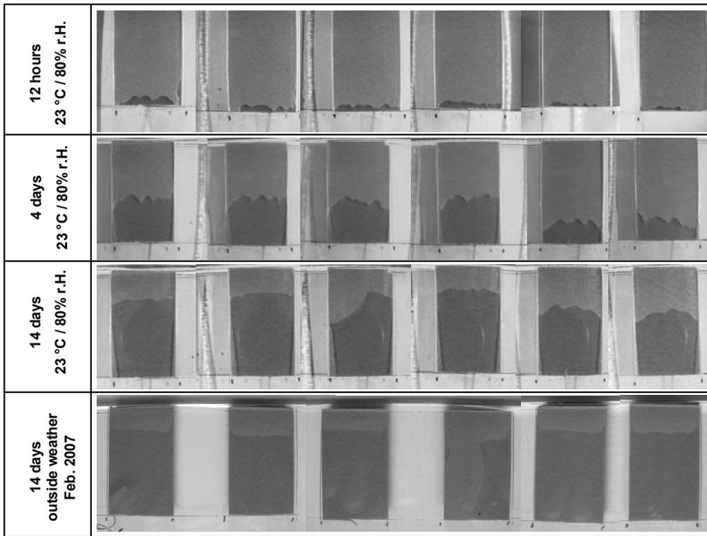
**Figure 10.** Test panels without primer, progress of debonding for different aging times and conditions
