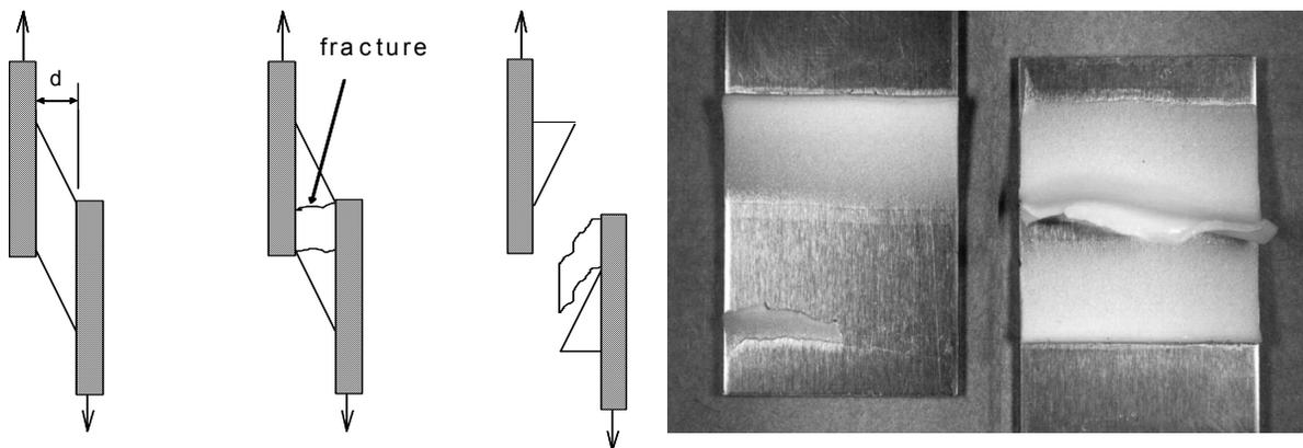
**Figure 6.** Bond failure under excessive shear due to cohesive fracture of the adhesive
