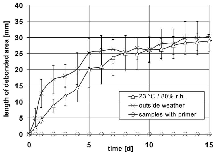
**Figure 11.** Time dependent average crack propagation length, average of six specimens
