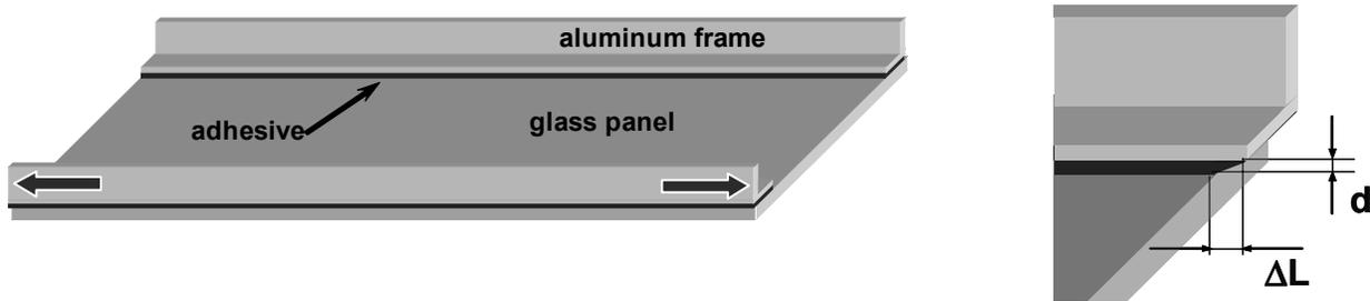
**Figure 2.** Shear strain at the edge of a bonded assembly due to thermal movement
