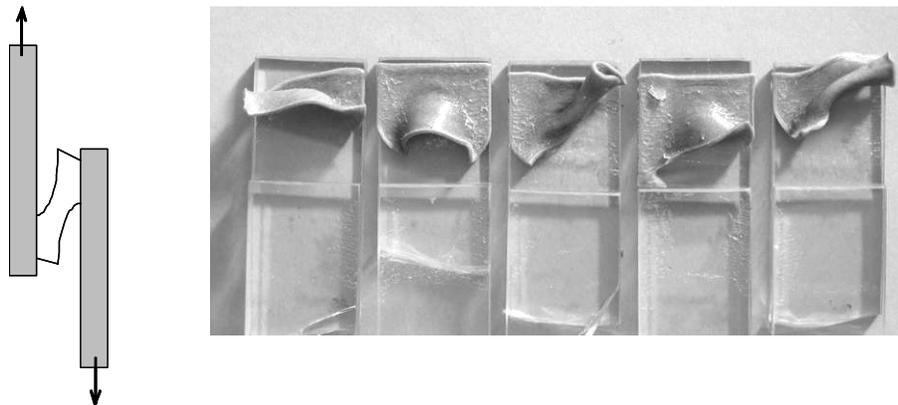
**Figure 7.** Failure of single lap shear specimen due to interfacial debonding after two weeks exposure to  $60^{\circ} \text{C} / 90\%$  relative humidity, float glass samples bonded with acrylic pressure sensitive tape
